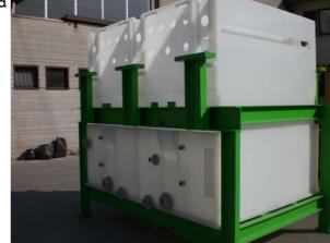
As it provided by the DVS 2205 norm any Chemical products storage tanks applied on waste water plants or other devices are designed and manufactured, out of PP or PE slabs. The focus point of these tanks is their absolute customizing possibility and their favorable quality / price ratio:
